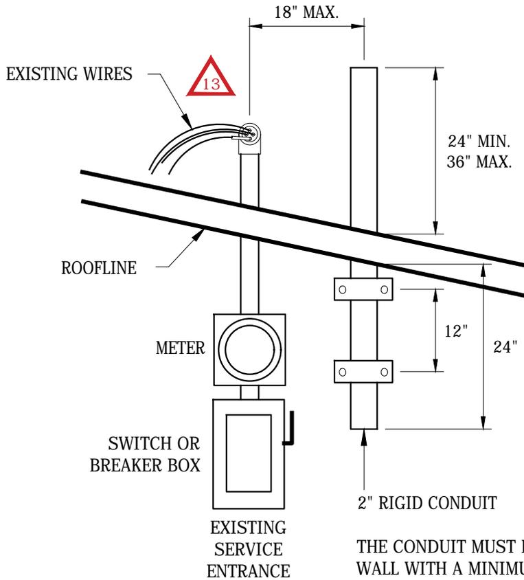
THE CONDUIT MUST BE FIRMLY SECURED TO THE WALL WITH A MINIMUM OF TWO 2-HOLE PIPE STRAPS ATTACHED WITH 1/4 INCH MINIMUM TOGGLE BOLTS OR 1/4 INCH MINIMUM LAG SCREWS IN LAG SHIELD ANCHORS
